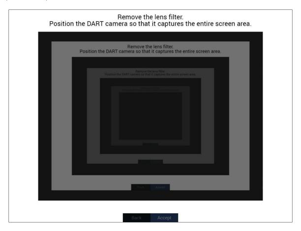
Position DART so that it completely captures the entire projected image. You can adjust the position of DART by loosening the tripod head and rotating the DART unit. Once the position is correct, tighten the tripod head. Once DART is positioned correctly, click the Next Step button to continue.
